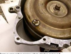
Torque converter access when starter removed
