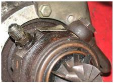
Turbocharger oil pipe connections
