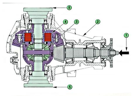
LSD using clutch plates<sup>1</sup>
