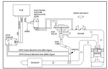
EGR system using differential pressure monitoring
