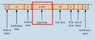
The data field is 64 bits which is 8 bytes
