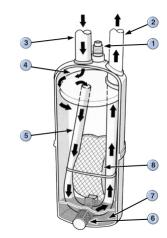
Low-pressure accumulator assembly<sup>1</sup>
