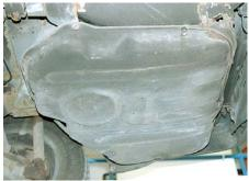
Fuel tank from under the vehicle
