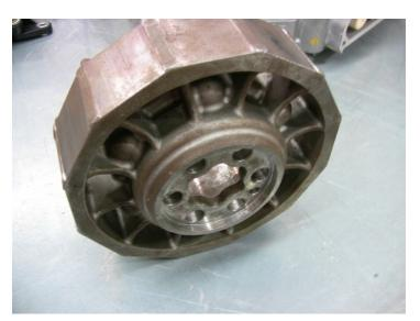
The core or rotor is made of very strong rare earth metal permanent magnets
