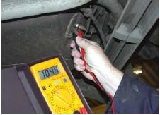
Testing at the tank unit
