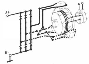
Alternator rectifier and current flow paths<sup>3</sup>
