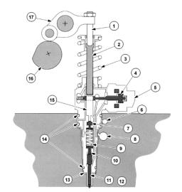
Design of the unit injector
