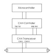
**Summary** A CAN message may vary between 44 and 108 bits in length. This is made up of a start bit, name, control bits, the data itself, CRC error detection, a confirmation signal and finally a number of stop bits.
