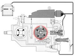
Bosch VR pump radial pistons
