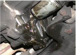
Checking the final drive output bearings and seals
