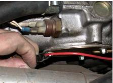
Electric manifold heating was used on some systems
