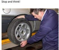
Checking the bearing freeplay
