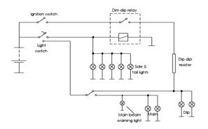
**Lighting circuit with a dim-dip relay fault** The symptoms of the fault on this circuit are that the dip lights are dimmed even when they are switched on fully. These symptoms should narrow down the fault (or faults!) but use the voltmeter to check exactly what the problem is.
