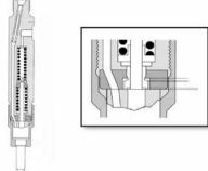
Two spring direct injection injector
