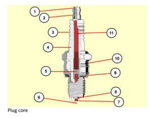
**Selection of the Correct Plug** The range of design details that are included in spark plug classification and identification are code letters or numbers for thread diameter, length of thread (reach), and design features such as radio suppression, taper seat and electrode type, the heat range, and the electrode gap. Special materials used in the construction of the plug are included in the manufacturer's name for the range of plugs or by a code letter in the identification classification.
