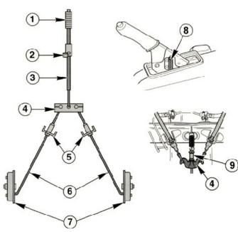
Parking brake mechanism<sup>1</sup>
