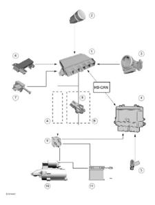
Example of a manufacturer's data (Ford): Keyless starting system 1-Keylesss vehicle module, 2-Start/stop button, 3-Electronic steering lock, 4-Powertrain control module, 5-Crank sensor, 6-Keyless vehicle antenna, 7-Vehicles with manual transmission: Clutch pedal position switch / vehicles with automatic transmission: Stoplamp switch, 8-The TR sensor, 9-Starter relay, 10-Starter motor, 11-Battery (Source: Ford Motor Company)
