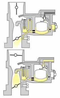
Carburetor metering fuel into the air stream
