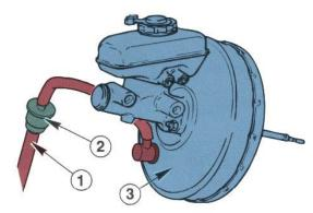
A check valve is fitted in the vacuum supply
