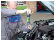
Float type hydrometers are the most accurate
