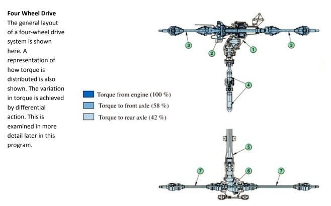
Torque distribution in a 4WD system<sup>1</sup>
