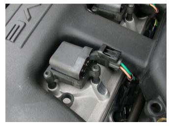
**Coil on plug (COP) or direct ignition 2** This screen shows connections to the high voltage coil spark plug outputs. A special adapter is often needed to make this connection. Check each cylinder in turn to see why this engine is misfiring.
