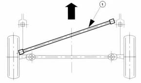
Panhard rod and torsion beam system<sup>1</sup>
