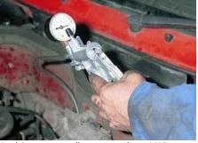
Applying a vacuum (low pressure) to a MAP sensor
