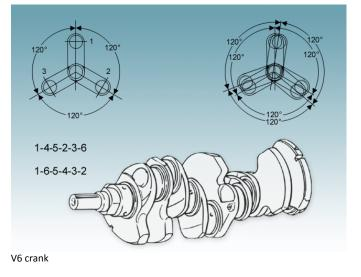
**V6 Cylinder Numbering** V-6 engines are numbered in two ways. One system numbers one bank with one, two and three and the other bank with four, five and six. The other numbering sequence uses alternate banks with one, three and five on one side and two, four and six on the other. Firing sequences are either one bank followed by the alternate bank or one cylinder from one bank followed by a cylinder from the other bank. These variations are shown in the accompanying diagrams.
