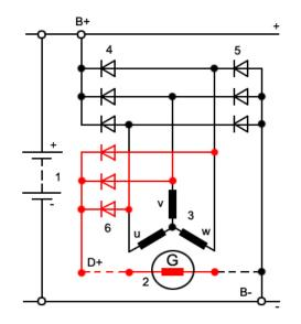
Field diodes and current flow to rotor and regulator<sup>3</sup>
