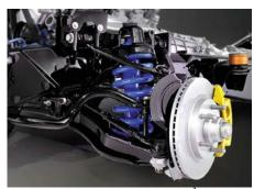
Twin, unequal length wishbone system<sup>2</sup>
