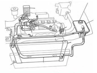
Liquid cooling system coolant flow
