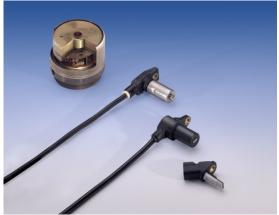
ABS wheel speed sensors (Source: Photo Bosch)
