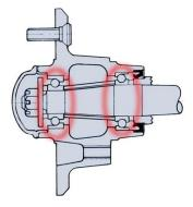
Front hub with tapered roller bearings
