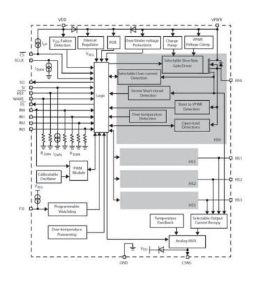
Internal configuration of an eXtreme or high side switch (Source: FreeScale)
