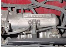
Inlet manifold plenum chamber
