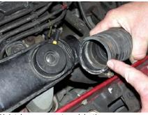
Air intake components and ducting
