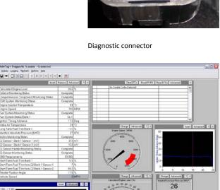
**Software** Running on a standard PC or laptop, the software allows the technician to choose which parameters or signals they want to see, and to view them as tables, graphs or gauges.
