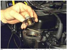
Thermostat with its wax pellet in the hot coolant area
