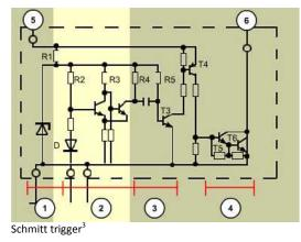
**Primary Current Cut-Off** Because the initial state of this circuit is with a zero output voltage, the ignition coil is not energized until the engine is rotating. The primary circuit is switched on by the first signal from the pulse generator with sufficient voltage to trigger the circuit.
