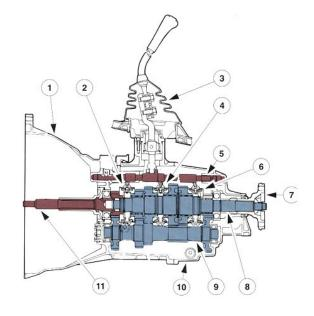
Sectioned view of a gearbox<sup>1</sup>
