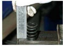
Checking the valve spring
