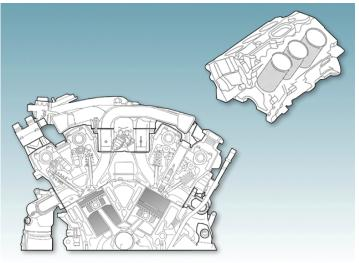
Dry liners are not in contact with the coolant
