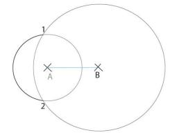
At a known distance from two fixed points 'A and B' you must be at position 1 or 2
