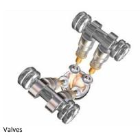
**The Four-Stroke Cycle (or Otto cycle**) The opening and closing of the valves and the movement of the pistons in the cylinders follows a cycle of events called the four-stroke cycle or the Otto cycle after its originator.
