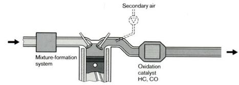
A catalytic converter system<sup>3</sup>
