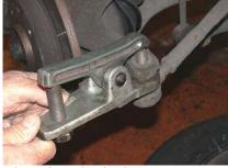
Splitting the track rod end joint
