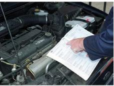
Check exhaust gas test results against data
