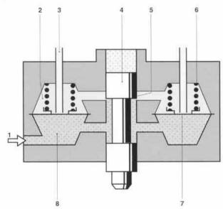
Differential pressure valve layout<sup>3</sup>
