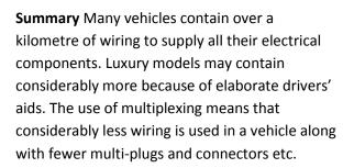
An additional advantage is that existing systems can be upgraded or added to without modification to the original system.
