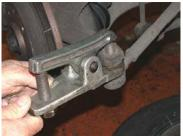
Splitting the track rod end joint
