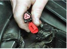
Checking the timing plug
