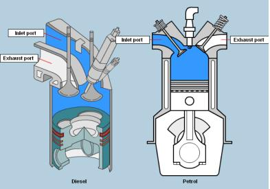
**Poppet Valves** The valves are 'poppet' and have a circular plate at right angles to a central stem that runs through a guide tube. The plate has a chamfered sealing face in contact with a matching sealing face in the port. The valve is opened by a rotating cam and associated linkage and closed and held closed by a coil spring.
