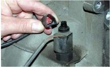
Cable drive and speed sensor assembly
