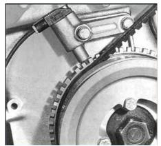
Inductive pulse generators on crankshaft pulley
