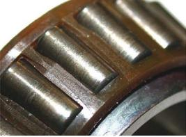
Damaged wheel bearing
