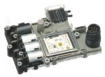
Electronically controlled valve block<sup>4</sup>
