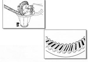
Braking the crown wheel / Ideal contact pattern<sup>1</sup>
