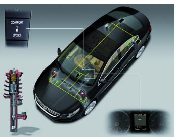
Active suspension also allows adjustments, in this case, between sport and comfort settings (Source: Volkswagen Media)
