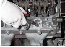
Clean the plug recess before removal
