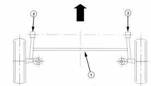
Torsion beams twist to provide the spring action<sup>1</sup>
