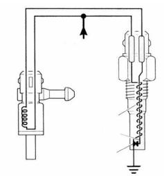
Cold start injector and circuit
