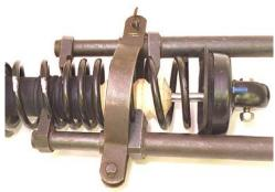
Coil spring in a compression tool
