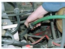
Pressure test and check under the heater
