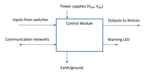
The basic central control system can be simplified in a way that is represented here
