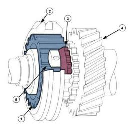
**Neutral Position** In the neutral position, the shift ring and blocker bars are centralized. There is no connection between the shift ring and the gear wheel. The gear wheel can turn freely on the shaft.
