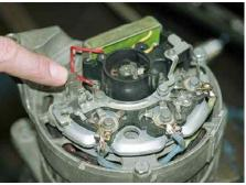
The rectifier must be removed for testing
