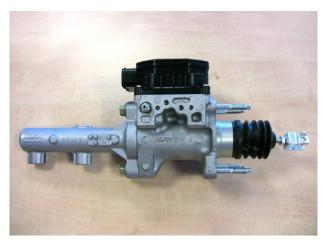
Electronically controlled brake master cylinder
