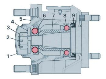
**Summary** The hub and bearing arrangement on the front of a front-wheel drive car must bear weight, withstand driving forces and support the driveshaft. The rear hub and bearings must support the vehicle and withstand side forces.
