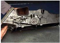
Heater box flaps must be set correctly
