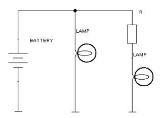
**Summary** This section has shown how simple voltage readings are used to determine faults on series and parallel circuits – remember that EVERY circuit on a vehicle is series or parallel – there are no other ways to do it!
