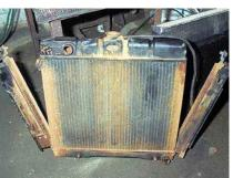
Sediment in the radiator may result in the need for serious repairs!
