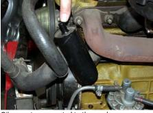
Oil separator connected to the crankcase
