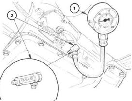
Pressure gauge connected<sup>1</sup>
