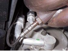
Heated exhaust gas oxygen sensor
