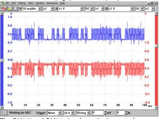
The CAN-H and CAN-L signals can be inspected as shown here on a PicoScope
