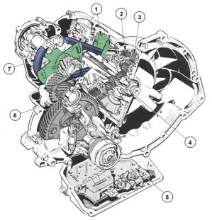
Drive Belt The key to this system is the high friction drive belt. The belt, made from high-performance steel, transmits drive by thrust rather than tension. The ratio of the rotations, or the gear ratio, is determined by how far the belt rides from the centers of the pulleys. The transmission can produce an unlimited number of ratios. As the car changes speed, the ratio is continuously adjusted.
