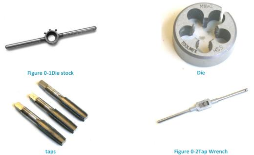
A tap cuts a thread on the inside surface of a hole, creating a female surface which functions like a nut. The three taps in picture show the three basic types:
