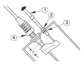
**Kick-Down Adjustment** Get an assistant to push the throttle pedal down slowly while you watch the throttle spindle and kick-down cable movement. Alternatively, move the throttle by hand from within the engine compartment. If the pull on the cable is incorrect, adjust the position of the outer sleeve until the movement is as specified. This is often a figure of 10 mm to 15 mm or about half an inch.
