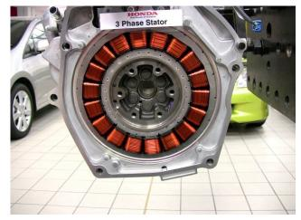
Motor stator in position on a Honda engine
