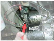
Meter connected to solenoid terminal
