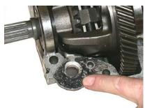
**Refit Final Drive – RWD** Clean off any old gaskets from the mating surfaces. Renew gaskets and use sealant as required. Refit the RWD final drive unit and torque the bolts in sequence. Refit the halfshafts, secure the halfshaft bearings, and fit the drums and wheels. Refit the propshaft. Finally, fill up with the correct oil.
