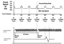
Detection of misfire by crank sensor signal
