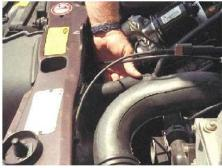
Engine must be up to temperature for a smoke test
