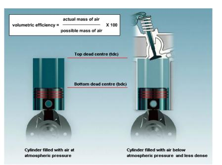
**Breathing or Aspiration** With a higher percentage, a greater quantity of air will be provided for expansion during combustion, and this improves performance. The intake and exhausting of air through an engine is known as 'breathing' or 'aspiration' and is important to produce efficient and clean combustion.
