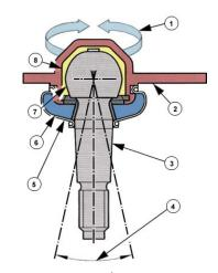
Ball joints are used instead of kingpins<sup>2</sup>
