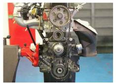
Camshaft belt and water pump drive pulley
