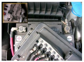
**Summary** Normal battery voltage is about 12.6V and when the engine is running, this should increase to about 14.2V. However, on some smart charging vehicles this can vary depending on conditions so as always, check manufacturers' data. Circuit voltage drop should usually be less than a few tenths of a volt.
