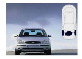
**Front engine RWD** Rear wheel drive from a front engine was the method used for many years. Some manufacturers have continued its use, BMW for example. A long propeller shaft from the gearbox to the final drive, which is part of the rear axle, is the main feature. The propshaft has universal joints to allow for suspension movement. This layout has some advantages.
