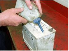
Water (H<sub>2</sub>O) is lost as H and  $O_2$  – only top up with distilled water
