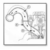
intake for diesel engine
