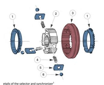
**Selector and Synchronizer** Most gearboxes have three synchronizers. Their task is to bring the chosen gear to the correct speed for easy selection. The unit consists of cone clutches to synchronize speed, and dog clutches to connect the drive.
