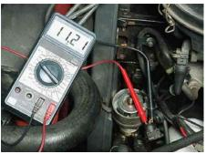
Checking Hall sensor supply voltage
