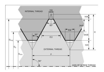
ISO Metric thread profile (the M10 in the given example refers to Dmax and the 1.5 refers to P)
