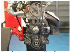
Camshaft belt and water pump drive pulley
