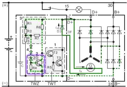
Rotor winding is switched on and off as a result of the zener diode conducting<sup>3</sup>
