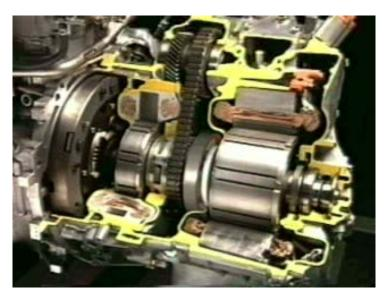
This cutaway shows the two motor/generators with the splitter and CVT in between (Source: Toyota)
