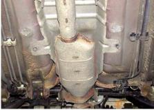
Catalytic converter heat shield
