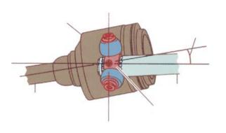
**Tripod Joint** The tripod joint is different from other constantvelocity joints. A component called a spider splits the drive angle. The arms of the spider give it the tripod name. Each arm of the spider has needle roller bearings and a roller ball. The roller balls work in grooves in the housing. This joint is suitable for inner or outer positions.
