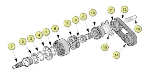
Transfer box using planetary gears and a drive chain<sup>1</sup>
