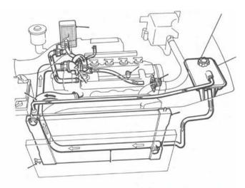
Liquid cooling system coolant flow
