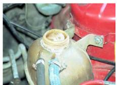
Expansion tank during back flushing
