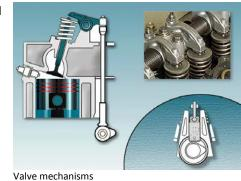
Overhead Cam (OHC) Layouts The term overhead cam distinguishes the position of the camshaft when it is fitted into the cylinder head. There are a number of single overhead camshaft (SOHC) positions using direct or rocker arm mechanisms to push onto the valve stems. These design variations have resulted from the need to maintain a close tolerance in running clearances.
