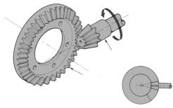
Bevel gears change ratio and drive angle
