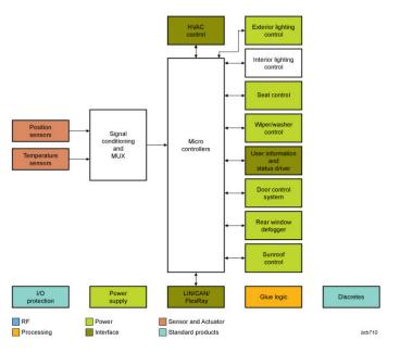
Central control module block diagram (Source: NXP)
