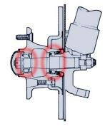
Front hub with tapered roller bearings
