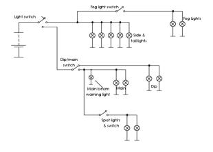
**Lighting circuit with a dim-dip relay** All the switches are in the position shown in red on this diagram and the circuit is operating correctly. Use the meter to take readings on this circuit and keep a note so you can compare them to those that you get on the next screen where a fault has been introduced.
