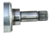
Splines on a driveshaft
