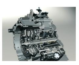
**Gear selection** 1<sup>st</sup>, 3<sup>rd</sup>, 5<sup>th</sup> and reverse gears are selected via multi-plate clutch 1. 2<sup>nd</sup>, 4<sup>th</sup> and 6<sup>th</sup> gears are selected via multi-plate clutch 2. One transmission unit is always in gear and the other transmission unit has the next gear selected ready for the next change, but with its clutch still in the open position.
