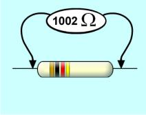
Testing a resistor
