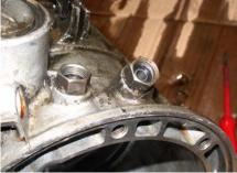
Oil cooler ports used for testing
