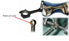
**Big-End Bearing** The big end is a split bearing mounting consisting of a forged fork in the rod and a matching cap. These are held together with studs or through bolts and nuts or with bolts threaded into the rod.
