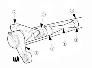
An anti-roll bar is a torsion spring<sup>1</sup>
