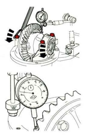
Turning the adjusting nut / Checking the backlash<sup>1</sup>
