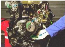
Lock pins hold the engine in position
