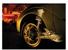
Suspension strut in position<sup>2</sup>
