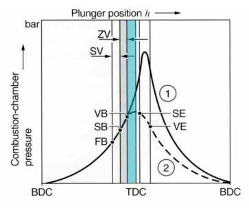
Controlled combustion in cylinder
