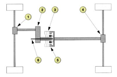
Viscous Coupling A viscous coupling is designed to transmit drive when the axle speeds differ. This occurs because the difference in speed of the two axles increases the friction in the coupling. This results in greater torque transmission, which in turn reduces the speed difference. As the speed difference reduces, less torque is transmitted. In this way, the torque is shared proportionally between the two axles.
