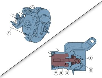
Sliding caliper parking brake<sup>1</sup>
