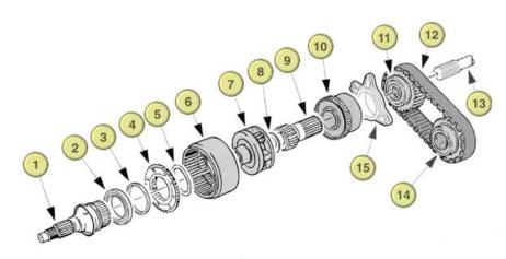
Transfer box using planetary gears and a drive chain<sup>1</sup>
