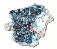
...showing coolant flow ports<sup>1</sup>
