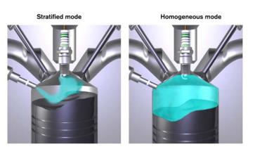
The injection point must be adjustable<sup>4</sup>
