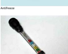
A hydrometer is used for testing antifreeze percentage
