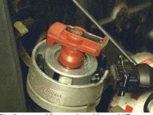
Distributor used for speed, position and HT switching
