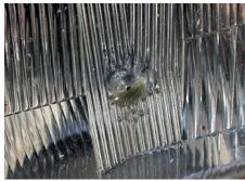
Damaged headlight lens
