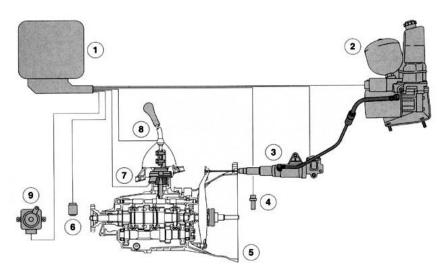
Electronically operated clutch<sup>1</sup>
