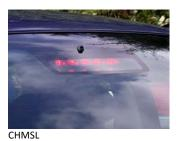
**Summary** Reverse lights are operated by a simple on/off gearbox switch. Brake lights are operated by a simple on/off switch on the pedal box. Both circuits operate in much the same way. High mounted brake lights are now quite common, and many of these use LEDs.
