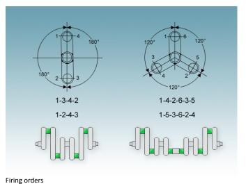
**V6 Big-End Journals** V-6 engine big-end journals carry two connecting rods each, with one from each bank of cylinders. The journals are positioned at 120° intervals and are either a single journal or splayed or offset journals with the two big-end crank pins offset in order to match the connecting rod angle to the journal.
