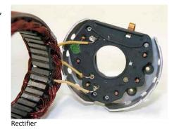
Half-Wave Rectification Rectification of alternating current (AC) to direct current (DC) is achieved in a rectifier by allowing a forward flow of current to pass through a diode, and then preventing the reverse flow from passing through. This simple method is called partial or half-wave rectification.
