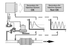
Secondary airflow diagnostic monitoring
