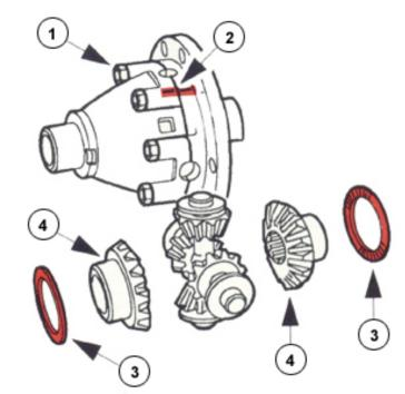
Differential bevel gears and thrust plates<sup>1</sup>
