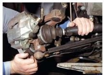
Removing the driveshafts
