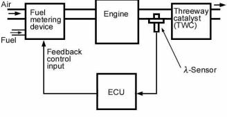
losed loop control sensors and connections
