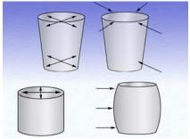
Exaggerated wear of a cylinder
