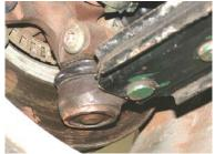
Greasing swivel joints is only necessary on older cars
