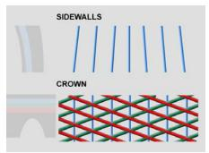
Sidewall and crown construction
