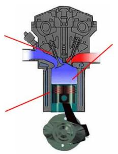
How oil gets in the combustion chamber
