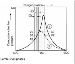
Phases of Diesel Fuel Combustion The most important phase of controlled combustion is when fuel is being injected into a burning mixture. This must be at a rate that maintains an even combustion pressure onto the piston throughout the critical crankshaft rotational angles. This gives maximum torque and efficient fuel usage, because temperatures remain controlled and the heat lost to the exhaust is minimised. The low temperatures also help to keep nitrogen oxide emissions (NOx) to a minimum.
