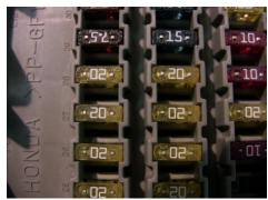
The multiplex control unit is incorporated in this fuse box
