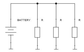
**Parallel circuit fault** This circuit has a problem. Take the readings again and you will notice that the voltage across one of the resistors is not correct. Check again and from the results, see if you can determine what is wrong. Click the 'A' button for the answer – and again, don't cheat!
