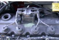
DIS coil and plug wires
