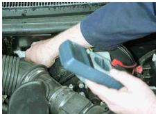
Testing the MAP sensor with a voltmeter
