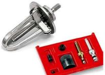
Internal and external bearing puller<sup>5</sup>
