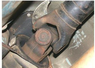
Rear driveshaft or propshaft
