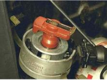
Check the output from a Hall sensor with a voltmeter or scope
