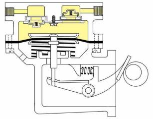
Operation of mechanical fuel lift pump
