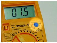
Transistor test socket on a multimeter
