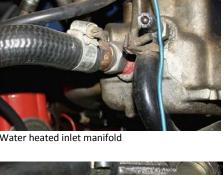
Water heated inlet manifold
