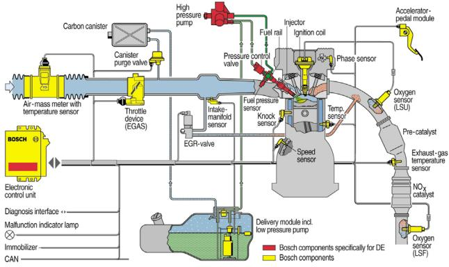
Exhaust gas oxygen sensors positioned pre and post catalyst (highlighted)
