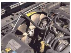
Viscous fan hub on a modern engine
