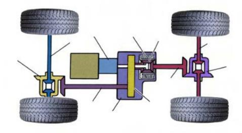
Differential fitted between front and rear axles
