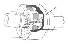
**Gaiter or Boot** The rubber boot or gaiter is to keep out the dirt and water and to keep in the lubricant. Usually a graphite or molybdenum grease is used, but check the manufacturer's specifications to be sure.
