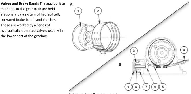
Brake bands lock different components<sup>1</sup>
