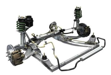
Advantages and disadvantages The main advantage of a conventional suspension system is its predictability. Over time the driver will become familiar with a car's suspension and understand its capabilities and limitations. The disadvantage is that the system has no way of compensating for situations beyond its original design. Jaguar suspension system (Source: Jaguar Media)
