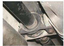
Propshaft center bearing mounting
