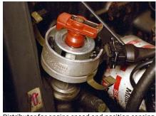
Distributor for engine speed and position sensing
