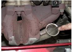
Pick up for hot air on an exhaust manifold
