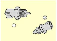
Coolant temperature sensors<sup>1</sup>
