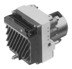
ABS and traction control modulator and ECU<sup>4</sup>
