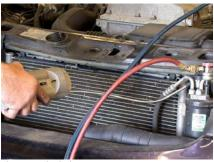
Electronic leak detector
