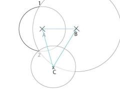
At a known distance from three fixed points 'A, B and C' then you must, in this case, be at position 2
