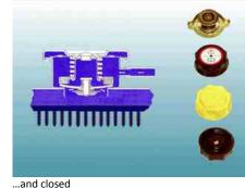
Bayonet and Ring Cap Fittings Bayonet fitting pressure caps are tightened on a ring cam under the lip of the filler neck. A safety stop is provided to prevent the cap from coming off. For removal, the cap has to be pushed down and turned to pass the safety stops. The cap should be turned fully clockwise when fitting to ensure the correct tension on the pressure release spring of the valve.
