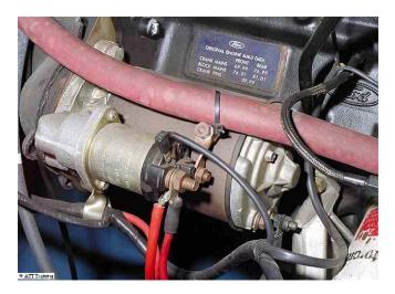
**Example fault 2** The symptoms of the fault on this circuit are that the starter is NOT cranking. Use the voltmeter to check exactly what the problem is.
