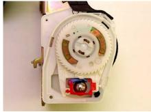
Seatbelt lock mechanism
