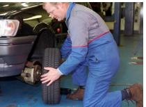
Wheel being removed ready for repair work
