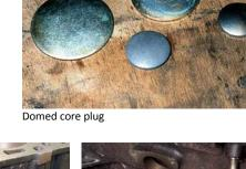
**Removal of Core** IPlugs Removal of the core plugs can be carried out using either a punch-through method or extractor method. Replacement is carried out using an appropriate size dolly and soft hammer. A hard-setting sealant is usually specified or recommended. It is smeared around the lip of the hole before fitting the core plug.
