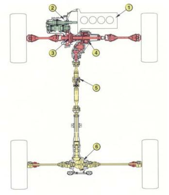
The main components of a four-wheel drive system<sup>1</sup>
