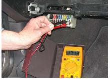
Ammeter reading motor current draw
