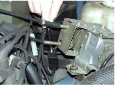
Checking the voltage supply to a valve
