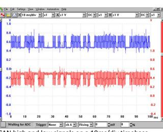
CAN high and low signals on a 10ms/div timebase (Source: www.picotech.com)
