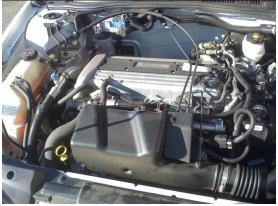
Figure 0-47 Natural gas converted engine
