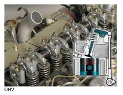
**OHV Valve Gear** The OHV valve gear consists of the camshaft, cam followers, push rods, and a rocker shaft or studs carrying rockers that push onto the valve stems.
