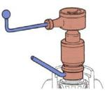
Setting the pinion preload and turning torque<sup>1</sup>
