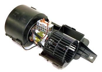
Typical motor and fan arrangement
