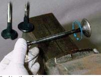
Checking the valve stem
