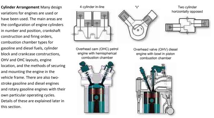
**Technical Details of 4-Cylinder 4-Stroke OHC Gasoline Engine** This diagram shows the components of this engine type. Look closely at the names and detail of these components before moving on to the next screens where they are shown individually with information on their purpose and construction detail.
