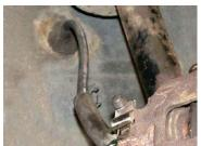
Check the flexible pipes
