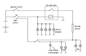
**Summary** A lighting circuit like any other, can be checked using a voltmeter. Remember, as a general guide, the circuit should always supply at least 95% of the battery voltage to the bulbs. Anything less than this indicates a high resistance and zero indicates an open circuit.
