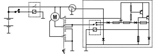
**Operation of the Circuit** De When either the delay contacts or the main switch contacts are operated, the motor will run at slow speed. When fast speed is selected, the third brush on the motor is used. Once switched off, the motor will continue to run until the park-limit switch changes over to the position shown. This switch is only in the position shown when the blades are in the parked position.
