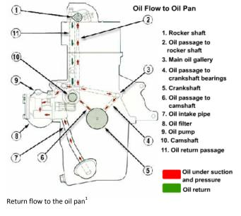
**Return to Oil Pan** The oil returning to the oil pan is directed through openings in the cylinder head and engine block so that it can provide an oil film for cleaning and protection of components. It is directed away from the shaft seals by throwers on the shafts and directed away from the crankcase ventilator (PSV) by suitably placed baffles and oil traps.
