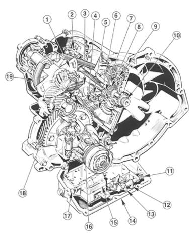
**Transmission Components** The main components of the CTX automatic transmission are shown here. Although the gear ratios are achieved through different means, the overall operation of the transmission is similar to other automatic types.
