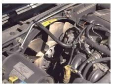
Viscous fan hub on a modern engine
