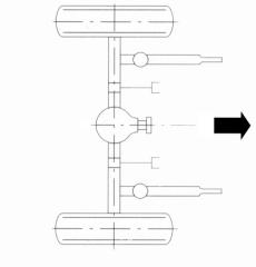
Welded compression/tension struts<sup>1</sup>
