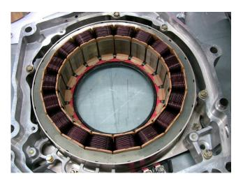
IMA motor stator removed from the vehicle
