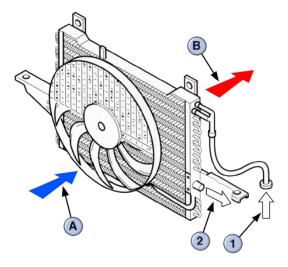
The condenser is very similar to the cooling system radiator<sup>1</sup>
