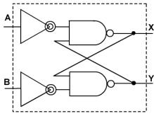
Basic memory building block made from gates
