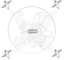
Four satellites used to determine vehicle position (Source: Ford)
