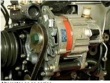
Alternator on an engine
