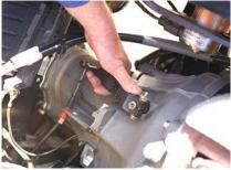
Remove the clutch cable
