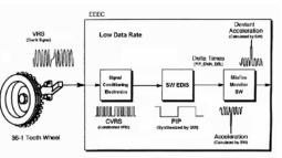
Crankshaft mounted wheel and sensor source of angular acceleration
