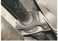
Propshaft center bearing mounting
