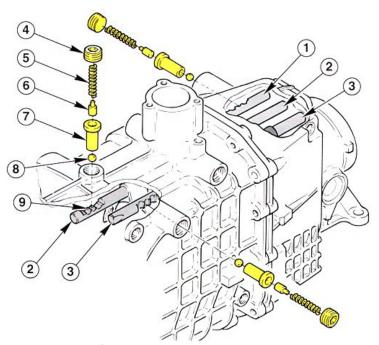
**Detent Mechanism** A detent mechanism is used to hold the selected gear in mesh. In most cases, this is just a simple ball and spring acting on the selector shaft(s). A gearbox with the detent mechanisms highlighted is shown here.
