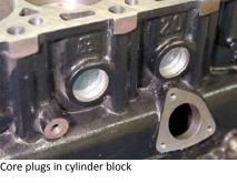
Core plugs in cylinder block
