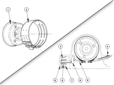
**Brake Band Movement** Oil pressure is used to actuate clutches and break bands. An actuator that tightens a brake band onto a rotating "drum" Is shown here. The drum, which in some cases is the outer side of the gear-set annulus, is stopped by the action of the brake band. This changes the ratio of the epicyclic gears.
