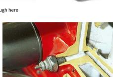
**Replacing Oil Pressure Switch** Refit or replace the switch with a light smear of thread sealant and reconnect the cable. Run the engine to test the operation.
