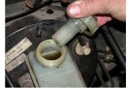
Checking the brake fluid level
