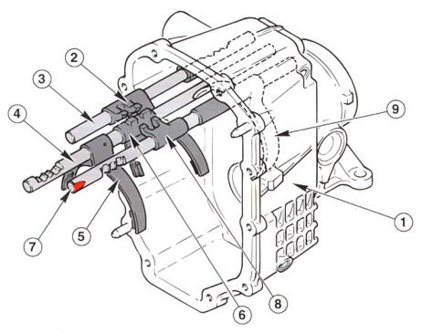
Three-Rail System The threerail, or three-shaft system, is similar to the two-shaft type. However, each shaft can be moved lengthways. In turn, the shafts will move the first/second, third/fourth or fifth/reverse forks.
