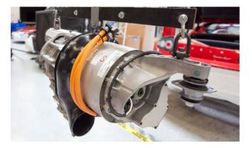
Figure 0-14 Tesla's AC induction motor (Source: Tesla Motors)
