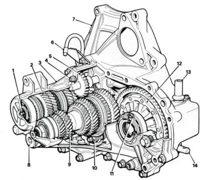
Internal view of a gearbox<sup>1</sup>
