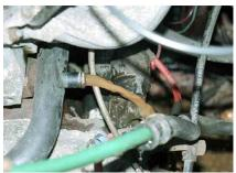
Reverse flushing the cooling system
