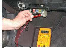
Testing a fuse in position
