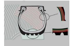
Plies embedded in layers of rubber
