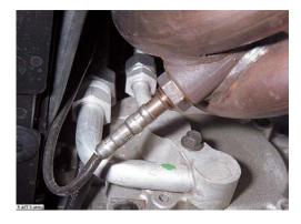
Figure 0-1 An exhaust gas oxygen sensor is one way to reduce emissions
