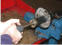
Testing a shock absorber off the car
