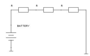
Series circuit fault This circuit has a problem. Take the readings again and you will notice that adding the readings across the resistors does not result in the battery voltage. This symptom indicates that there is a fault. Check the readings again and then see if you agree with the answer which will show if you click the 'A' button – and don't cheat!
