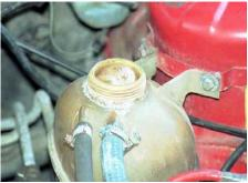
Expansion tank during back flushing
