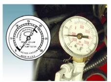
Vacuum gauges can be used to test the PCV system
