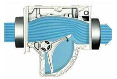
Action of the vane airflow meter<sup>3</sup>
