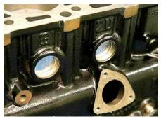
Engine block with core plugs
