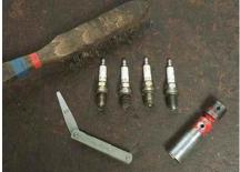
Keep plugs in order when removed for easy inspection
