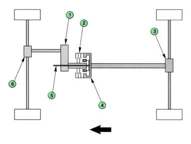
Power flow with a 4WD configuration<sup>1</sup>
