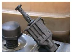
Alarm switch-type sensor
