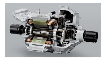
Figure 0-32 induction drive motor, differential and final drive components (Source: Honda Media)
