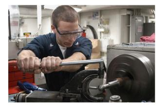
Repairs using lathe (Source: Wikimedia)
