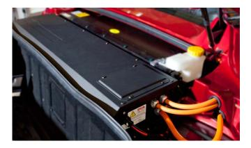
Figure 0-16 Power electronics module
