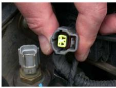
Connect a resistor in place of the temperature sender
