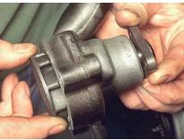
Checking water pump bearings
