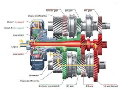
Output shaft 1 Located on output shaft 1 are:
