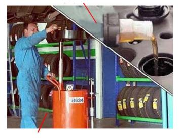
**Oil Condition** Looking at the condition of the oil will indicate the existence of problems that may be developing. Black oil can be caused by either a late oil change or could show early signs of piston blow by. Creamy or emulsified oil indicates the existence of water. Report any abnormality to the owner or driver of the vehicle.
