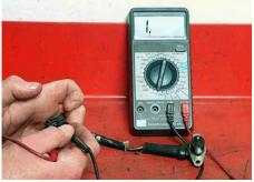
Engine speed sensor resistance measurement (faulty sensor)
