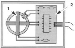
Field sensor: 1, crossed coils. 2, control circuit (Source: Ford) All GPS units must have some sort of compass
