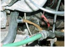
Reverse flushing the cooling system
