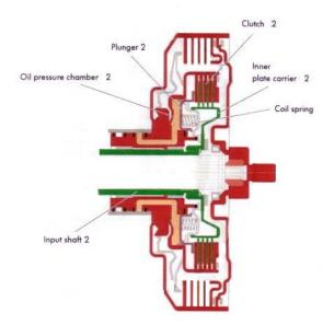
**Input shaft 2** Input shaft 2 is shown in relation to the installation position of input shaft 1. It is hollow and is joined via splines to multi-plate clutch 2. The helical gear wheels for 6<sup>th</sup>, 4<sup>th</sup> and 2<sup>nd</sup> gear can be found on input shaft 2. For 6<sup>th</sup>, 4<sup>th</sup> and 2<sup>nd</sup> gear, a common gear wheel is used. A pulse wheel is used to measure the speed of input shaft 2. The sender is adjacent to the gear wheel for 2<sup>nd</sup> gear.
