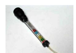
A hydrometer is used for testing antifreeze percentage
