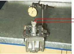
DTI used to check end float
