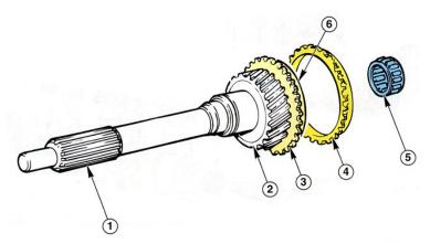
Details of the input shaft<sup>1</sup>
