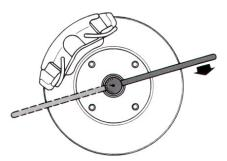
Checking the viscomatic lock<sup>1</sup>
