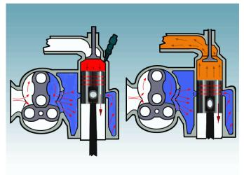
Diesel two-stroke cycle
