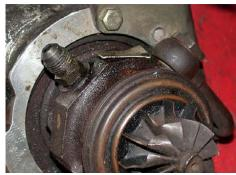
Oil pipe connections to the turbocharger
