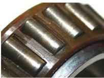
Damaged wheel bearing
