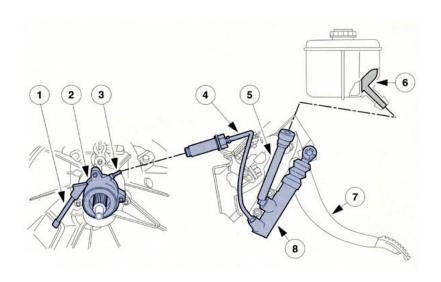
Clutch hydraulic components<sup>1</sup>
