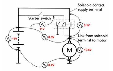
Starter circuit showing good voltmeter readings
