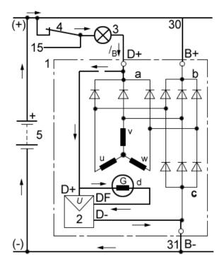
Internal and external alternator circuit<sup>3</sup>
