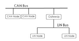
**Standard** The LIN standard includes the specification of the transmission protocol, the transmission medium, the interface between development tools, and the interfaces for software programming. LIN guarantees the interoperability of network nodes from the viewpoint of hardware and software, and predictable electro-magnetic compatibility (EMC) behaviour.
