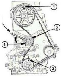
Timing Marks The engine must be correctly timed so that the valve opening and closing and the ignition spark occur at the correct points in the four-stroke cycle. Marks are provided on the engine and the belt pulleys, which must be aligned before the belt tension is released and the belt removed. The engine must be brought up to the timing marks in the normal direction of rotation of the engine to avoid setting to 'one tooth out' on the slack side of the belt.
