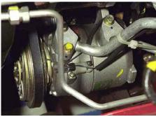
Air conditioning compressor and pipes
