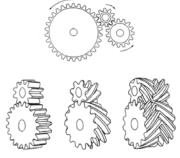
Straight cut and helical gears
