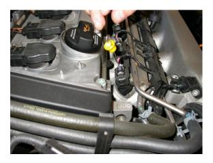
Test the voltage by back probing a connector with care
