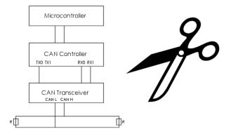
CAN nodes can be disconnected by the control program
