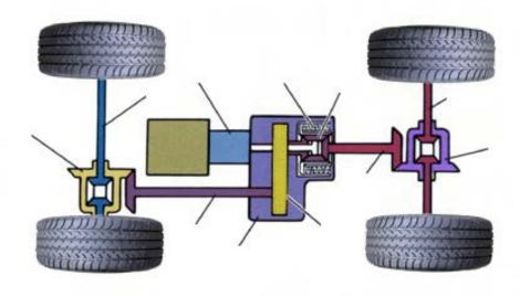
Differential fitted between front and rear axles
