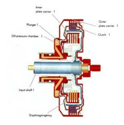
**Multi-plate clutch 2** Clutch 2 is the inner clutch and transmits torque into input shaft 2 for 2<sup>nd</sup>, 4<sup>th</sup> and 6<sup>th</sup> gear. As with clutch 1, oil is forced into the pressure chamber so that plunger 2 then joins the drive via the plates to input shaft 2. The coil springs press plunger 2 back to its start position when the clutch is opened.
