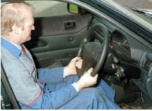
Checking operation of the gauges
