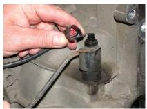
Speed sensor and cable connection
