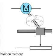
Electric Mirrors Many vehicles allow electrical adjustment of mirrors, particularly on the passenger side. The system is much the same as that used for seat movement. Two small motors are used to move the mirror vertically or horizontally. Many mirrors also contain a small heating element on the rear of the glass. This is operated for a few minutes when the ignition is first switched on. The circuit shown here includes feedback resistors for position memory.
