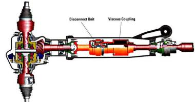
DU positioned in the transmission <sup>ZF</sup>
