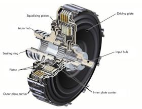
**Multi-plate clutch 1** Clutch 1 is the outer clutch and transmits torque into input shaft 1 for the 1<sup>st</sup>, 3<sup>rd</sup> 5<sup>th</sup> and reverse gear. To close the clutch, oil is forced into the pressure chamber. Plunger 1 is therefore pushed along its axis and the plates of clutch 1 are pressed together. Torque is then transmitted via the plates of the inner plate carrier to input shaft 1. When the clutch opens, a diaphragm spring pushes plunger 1 back into its start position.
