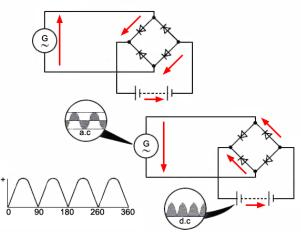
Bridge rectifier showing full wave rectification
