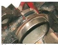
Caliper piston seal
