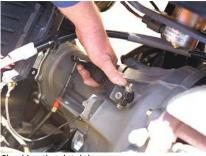
Checking the clutch lever
