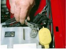
Battery earth lead being removed
