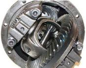
Crown wheel/Ring gear and differential
