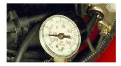
**Vacuum Readings** Vacuum is measured in inches or millimeters of mercury or in the SI unit of kilopascals (kPa). Two series of tests are made, one with the engine cranking, and the other with the engine running. During cranking a fluctuation of the needle occurs. If the swing is irregular it indicates problems with one or more cylinders, which would require a leakage or compression test to identify.
