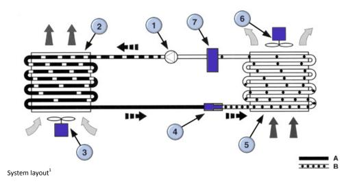
**High-Pressure Liquid** As the compressor operates, it causes the pressure on its intake side to fall. This allows the refrigerant in the evaporator to evaporate and draw heat from the vehicle interior. The high-pressure or output side of the pump is connected to the condenser. The pressure causes the refrigerant to condense, in the condenser, thus giving off heat outside the vehicle as it changes state.
