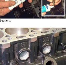
Core plugs in cylinder block
