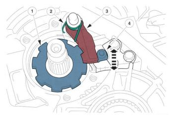
Locking mechanism for parking<sup>1</sup>
