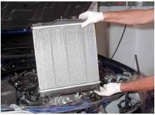
Lifting out radiator with electric fan and cowl
