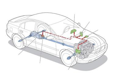
**Summary** Four-wheel drive systems use a combination of propshafts and driveshafts together with viscous couplings and transfer boxes. A number of variations are possible. These are described as full-time or part-time.
