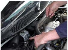
The cable runs along the bulkhead on this car
