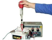
Testing a battery on charge
