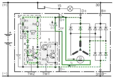
Regulator circuit - not conducting<sup>3</sup>
