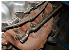
Air pipes in the exhaust manifold
