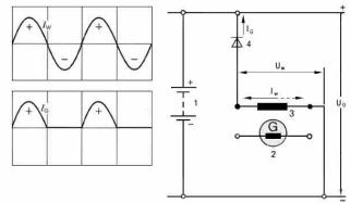
Simple diode controlling AC current flow to give half wave rectification<sup>3</sup>
