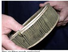
This air filter needs replacing!
