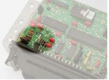
Resistors in an electronic control unit
