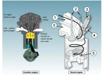
**Inlet Valve** The inlet valve remains open after the piston has reached bottom dead center (bdc) and has begun to move toward top dead center (tdc) on the compression stroke. The amount of piston movement is small as the crankshaft swings across the 180<sup>°</sup> position when the piston is at bottom dead center (bdc). The 'valve lag' allows the momentum of the incoming air charge to force a little more air into the cylinder even though piston movement is reducing the cylinder volume
