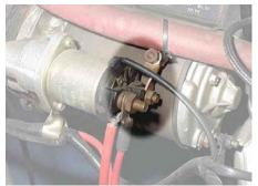
Solenoid to motor connecting strap
