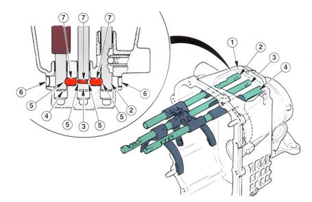
Sliding Plunger Interlock When three rails are used to select the gears, plungers or locking pins can be used. These lock the two remaining rails when one has moved. In the neutral position, each of the rails is free to move. When one rail (rod or shaft) has moved, the pins move into the locking notch, preventing the other rails from moving.
