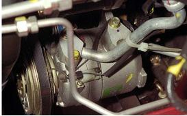
Compressor in place on the engine
