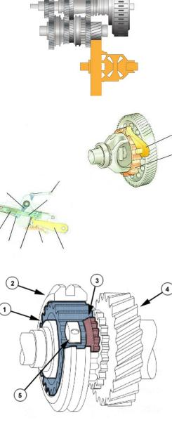
**Synchronisation 2** 1<sup>st</sup>, 2<sup>nd</sup> and 3<sup>rd</sup> gears are equipped with three-fold synchronisation. Compared with a simple cone system, a considerably larger friction area is provided. Synchronisation efficiency is increased as there is a greater surface area to transfer heat. This threefold synchronisation consists of:
