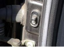
Switch positioned in the door pillar
