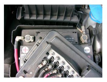
**Charging voltage** The engine is now running, at about 3000 rev/min. Check the voltage and note the reading. Click 'A' for my interpretation.
