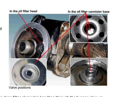
**Oil Flow Through Filter** The resistance to flow through a clean filter element is less than through the bypass valve, so normal oil flow is through the element. When the filter is blocked and the bypass valve opens the oil is no longer being filtered, so dirty oil may enter the engine. Some manufacturers fit an electrical warning lamp circuit with a switch fitted to the bypass valve.
