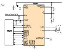
System basis chip (SBC) with a LIN transceiver. (Source: Freescale Semiconductor)
