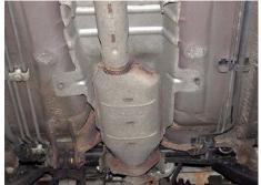
Catalytic converter on a vehicle
