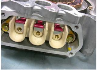
Motor terminals for the high voltage cables (which always have an orange covering)
