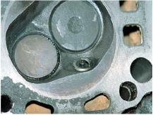
Spark plug from inside the engine
