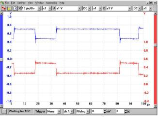
CAN high and low signals on a 10us/div timebase (Source: <u>www.picotech.com</u>)
