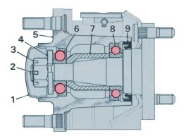
**Rear Bearings** The stub axle, which is solid-mounted to the suspension arm, fits in the center of two bearings. The axle supports the weight of the vehicle at the rear, when still or moving. Ball bearings are used for most vehicles with specially shaped tracks for the balls. This is so the bearings can stand side loads when turning. A spacer is used to ensure the correct distance between, and pressure on, the two bearings.
