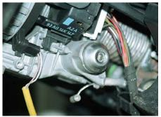
Switch connections under the steering cowling
