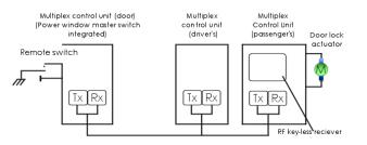
Bus-type (bi-directional) communication system using microcomputer-based communication ports
