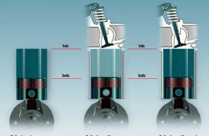
Cylinder at atmospheric pressure maximum mass of air Cylinder with poor volumetric efficiency has low pressure and low mass of air Cylinder with good volumetric efficiency has high pressure and good mass of air
