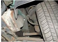
Coil spring from under the car
