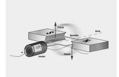
Direct current motor operating principle
