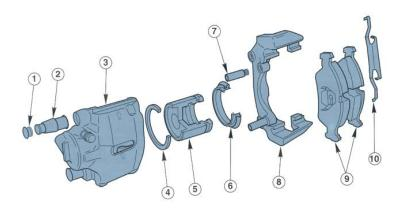
Sliding disc brake caliper components<sup>1</sup>
