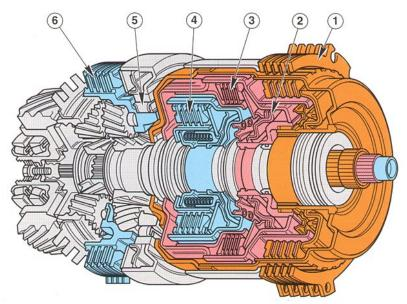
**Clutch Unit** The clutch unit consists of three multi-plate clutches, two multi-plate brakes and a roller one-way clutch. The appropriate clutches or brakes are supplied with pressure by the transmission module according to the selected drive range and shift program. The required components are driven, locked or allowed to rotate freely to select the different transmission ratios. The clutch unit acts on the components of the planetary gear train.
