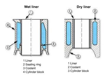
**Dry Liners** Dry liners are either fitted into the casting mold and held in place by the shrinkage of the casting (providing an interference fit), or they are pressed into a pre-cast block. The cast in types can usually be rebored whereas the pressed liners can be replaced.
