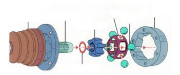
**Cross-Groove Joint** The Rzeppa joint is one of the most common. It has six steel balls held in a cage between an inner and outer race inside the joint housing. Each ball rides in its own track on the inner and outer races. The tracks are manufactured into an arch shape so that the balls stay in the midpoint at all times, ensuring that the angle of the drive is bisected. This joint is used on the outer end of a driveshaft. It will handle steering angles of up to 45 degrees.
