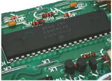
Microprocessor (microcontroller in this case)
