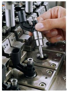
njector for direct injection under test<sup>4</sup>
