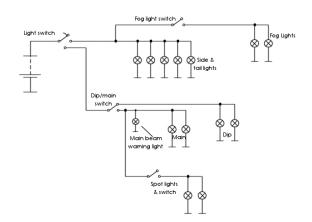
**Basic lighting circuit fault** The symptoms of the fault on this circuit are that the side, fog, spot and dip lights work correctly but the main beam lights are both dim. The main beam warning light does not come on. These symptoms should narrow down the fault (or faults!) but use the voltmeter to check exactly what the problem is.
