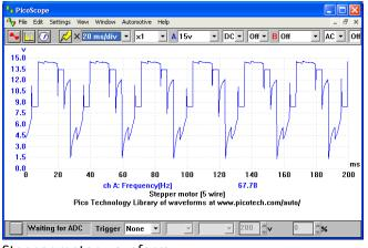
Stepper motor waveform
