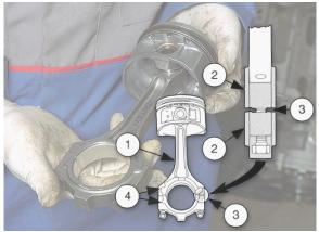
Details of the con rod and piston pin
