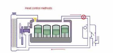
Heat control flap in heater housing Heater water valve plunger type Cold air vent Air heated as it  $\bigcirc$ passes through heater radiator
