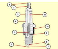
Spark plug in cross section
