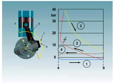
Gasoline engine figures – Diesel figures are approximately double
