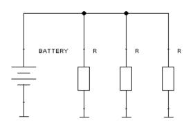
**Series-parallel circuit** Circuits on a vehicle are a combination of series and parallel as represented in a very simple way here. Take the readings with the voltmeter and see if they agree with the ideas we developed in the earlier screens. Click 'A' for my answer.
