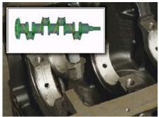
Drillings in the block and crank
