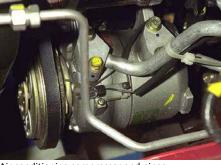
Air conditioning compressor and pipes
