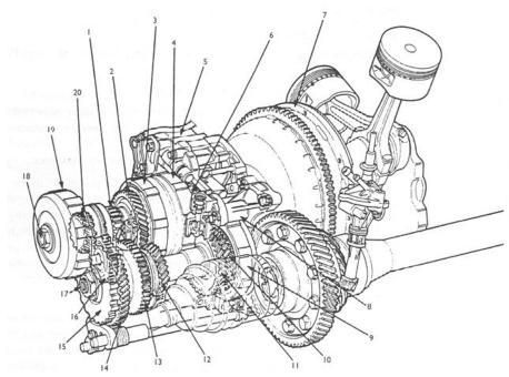
Standard Gear Systems Many automatic transaxle gearboxes use gears the same as in manual boxes. The changing of ratios is similar to the manual operation except that hydraulic clutches and valves are used. An example of this system is shown here.
