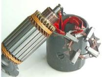
Armature and field coils
