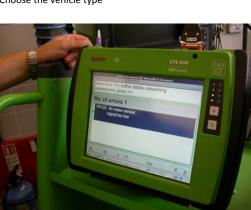
Take a readout from the control unit memory (DTC
