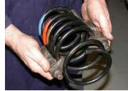
Coil spring removed from the strut
