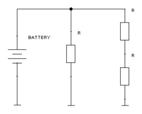
Series-parallel circuit fault Let's assume that in this circuit the resistor R represents an instrument panel dimmer control. The symptoms here are that the first lamp seems to light correctly but the second one does not dim, it is at full brightness. Take the readings to determine the fault – click 'A' for my answer.
