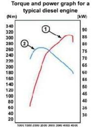
1 Power curve 2 Torque curve
