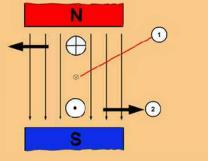
Magnetic forces reacting to give rotary motion
