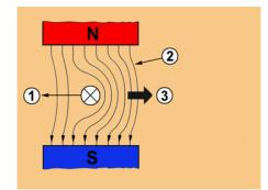
Electric current through a conductor in a magnetic field
