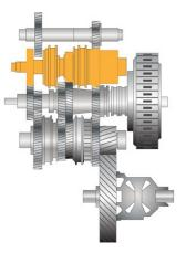
**Reverse shaft** The reverse shaft changes the direction of rotation of output shaft 2 and therefore the direction of rotation of the final drive in the differential. It engages in the common gear wheel for 1<sup>st</sup> gear and reverse gear on input shaft 1 and the selector gear for reverse gear on output shaft 2.
