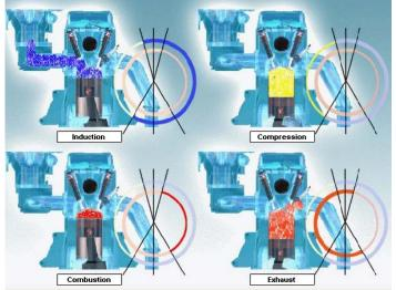
Four-stroke cycle and valve timing data
